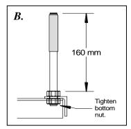
2. Set ragbolt into position, encapsulating the service pipes (and sullage branch if applicable), and pour concrete pad.
